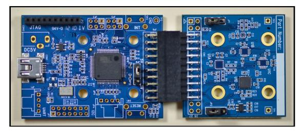
Figure 4. UEVB connected to InvenSense ARM Controller Board
