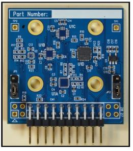
Figure 2. Top Side of the UEVB (e.g. MPU-65xx)
